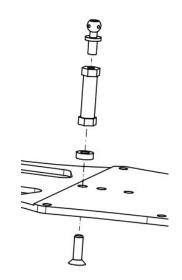
Using an HW033 M3x10 countersunk fix the screw FX0053-20 post. Install the 2mm shim between the post and the chassis. Tight the group firmly. Insert the male stud FX0061-M in the post.
