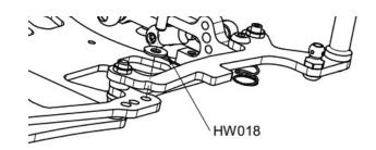
You can insert 1 x HW003 M3x8 button screw plus 1 HW018 M3 washer
