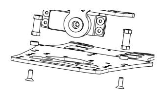
Using 2 x HW008 M3x6 Button, fix the servo group to the G12-7 servo holder.
