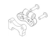
Secure the G56-030 upper arm mount to the G56-039 using 2 HW004 M3x10mm Hex button screw.
