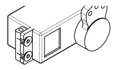
Assembled group. Servo saver should be vertical when servo is neutral.
