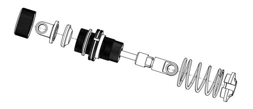
Close the shock absorber with rubber seal, ball joint and cap.
