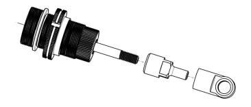
Screw together the G12-K7 droop adjuster and the ball joint (long one)
