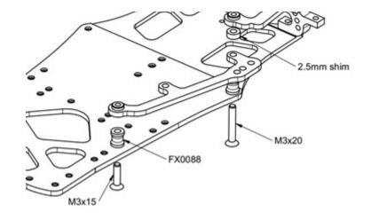
Install the side group as shown using 1 x HW001 M3x20 countersunk screw and 1 HW020 M3x15 countersunk screw.
