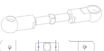
Build 2 set of link using 2 x TR15 and 4 FX0037 - short Keep this dimensions. Fix the link over the Vlink F2
