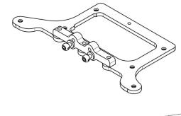
Insert 2 x male ball stud into the V-link F2.
