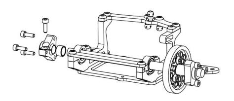
Fix the spur to the spool with the M3x6 screws.
