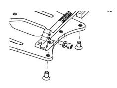
Assembly the M20 V-link1 to the chassis, using 2 x HW012 M3x6 countersunk screw.
