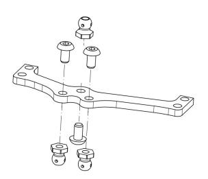
Insert the bearing into the G12-C bearing holder. Note that the mark should be on the same position (vertex NOT important) . G12-C allow you play with the wheelbase giving +1mm
