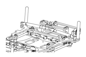
Install the G122-4 shock holder, using 4 by HW008 3x6 button screw
