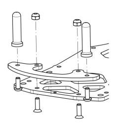
Install the front body post to the bumper using 2 x HW003 M3x8 button screws.
