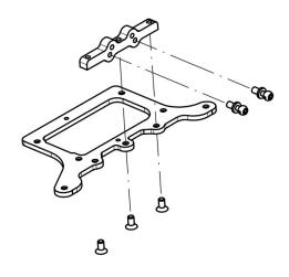
Using 3 x HW012 M3x6 countersunk screw fix the V-link F2 to the motor pod.
