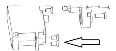
Enlarge the highlighted holes at 3mm diameter
